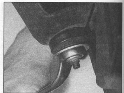
9.4 . . . then unscrew the lower mounting nut, and recover the washers and mounting rubber
