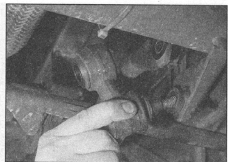
7.4b . . . and remove the connecting link from underneath the vehicle
