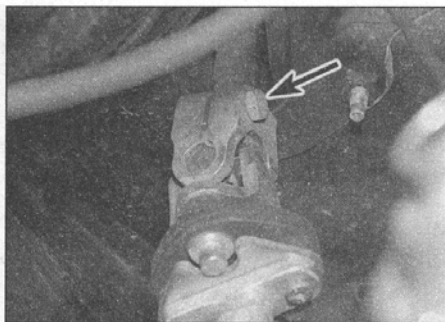
21.3 Intermediate shaft-to-steering column clamp bolt (arrowed)
