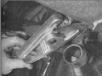
16.4b ... then use a universal balljoint separator ...
