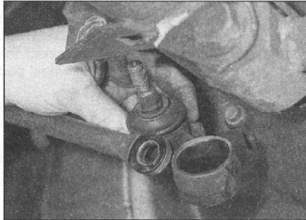
16.4c ... to free the connecting link from the axle
