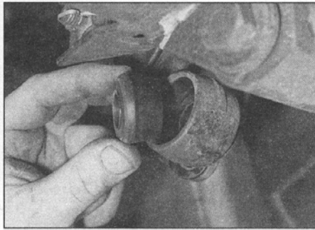
16.3c If they are loose, remove the mounting rubbers from the connecting link
