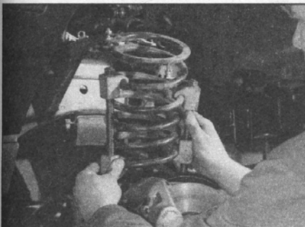
3.4a Remove the front coil spring . . .
